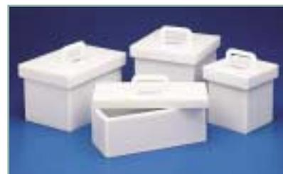
lead. This storage system is excellent for storing vials of isotopes, contaminated instruments and tools, radioactive samples, solutions or waste. A .76mm (.030") thick lead shield encased in 6.4mm (1/4") thick high-density polyethylene helps contain radiation without lead exposure. Each box has a cover of the same lead/polyethylene construction. The external lip has a 32mm (1 1/4") overlap designed to prevent radiation escape. The handle is 89 x 29mm (3 1/2 x 1 1/8") inside the lifting loop.
